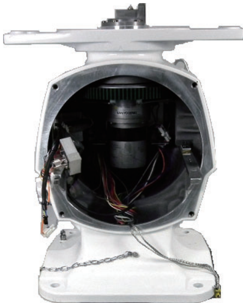
Rear view with cover and transceiver module RTR-101 removed.
