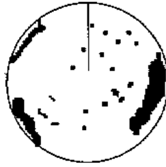
A/C RAIN control adjusted
