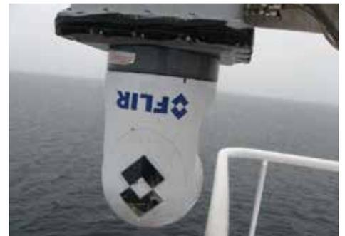
On both vessels the FLIR M-625XP thermal imaging cameras have been mounted in the "ball down" position.
